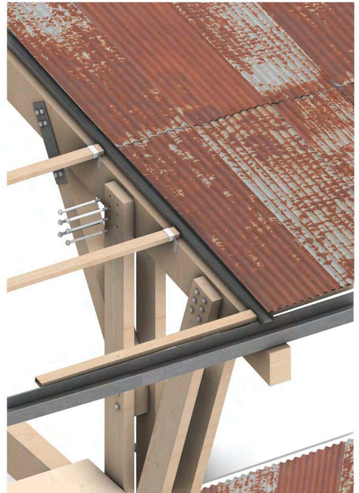
Roof and hidden gutter structure
